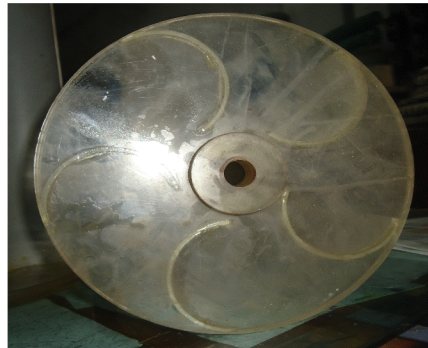
Figure 3: Cross-sectional view of five bladed rotor
